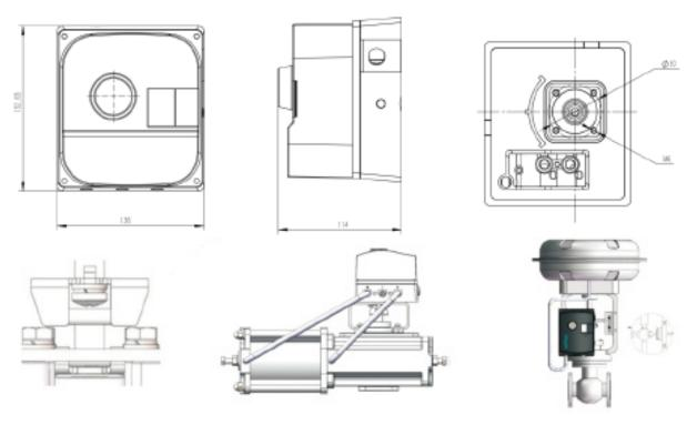
Mounting options include bracket mount and direct mount for rotary and in-line linear valves
